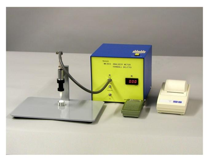
MK-201 Pressure Analgesy Meter has been designed for rapid and precise screening of analgesic drugs on the normal and inflamed rat paw according to the Randall-Selitto test and displays the pressure digitally.
