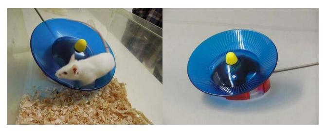
MK-713/CU01 IGLOO FAST-TRACS, Low-Cost Running Wheel is designed to measure spontaneous activity Levels of mice accurately. The plastic wheel is equipped with a sensor which detects the revolving of the wheel. As the wheel is mounted on the igloo (dome-shaped house) located in a home cage, it is easier for mice to run.
